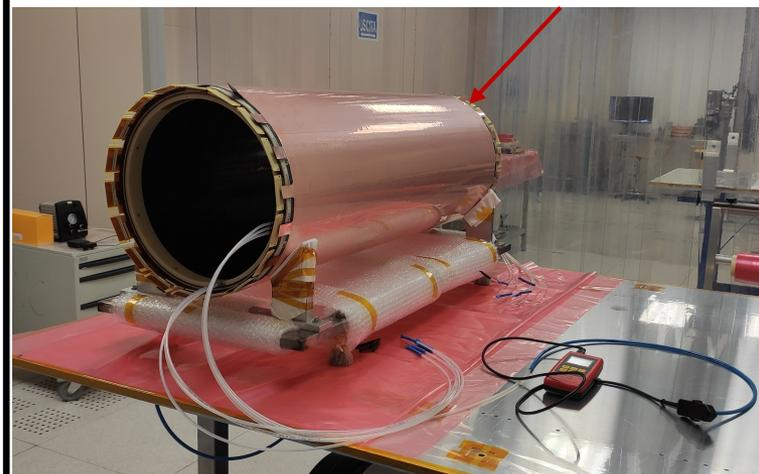
The first test showed a leakage
