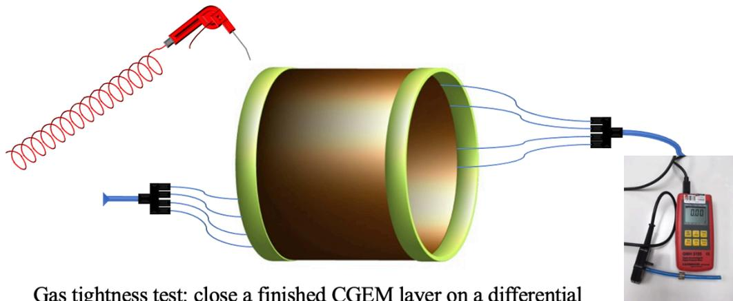
Gas tightness test: close a finished CGEM layer on a differential pressure meter, and blow  $N_2$  on the surface. If the  $N_2$  flow enters a hole, the instrument shows a sudden increase ( $\approx 0.1-1$  mbar) of the detector internal pressure wrt the atmospheric one.
