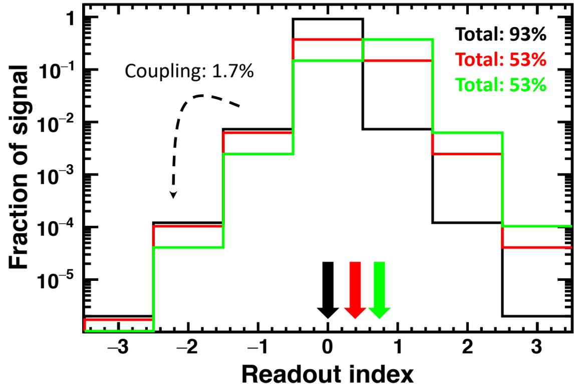
**Energy loss:** amount of signal lost for energy deposit in between strips with respect to readout ( $\sim 57\%$ ).
