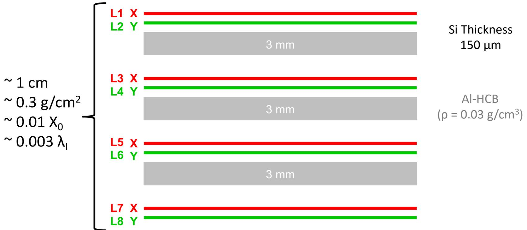
All geometry (number of planes, thicknesses, gaps, support structures) are decided in production.
