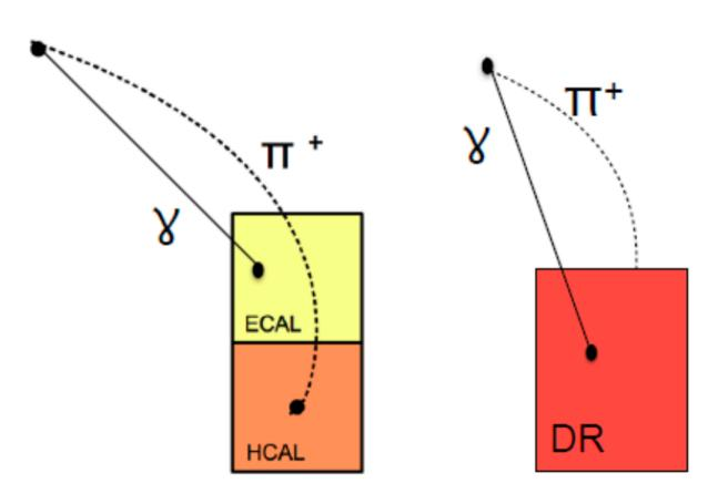
DR CAL module in Delphes assumes that it is always possible disentangle if a hit in the calorimeter cell is a charge only or charges + neutral hypothesis
