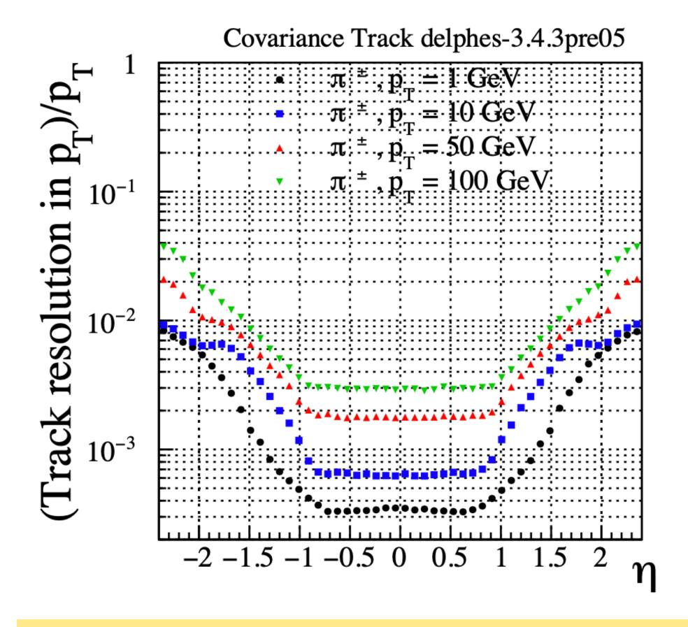
Expected variations of the resolutions in the barrel and forward region due to the different sub-detectors and layers crossed
