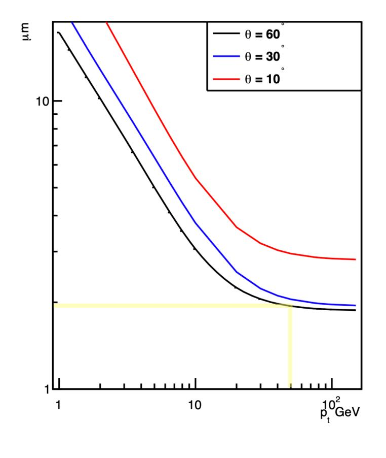
$\sigma_{d_0} \approx 2 \, \mu \mathrm{m}$  for particles with  $p_T \in [90-100]$  GeV
