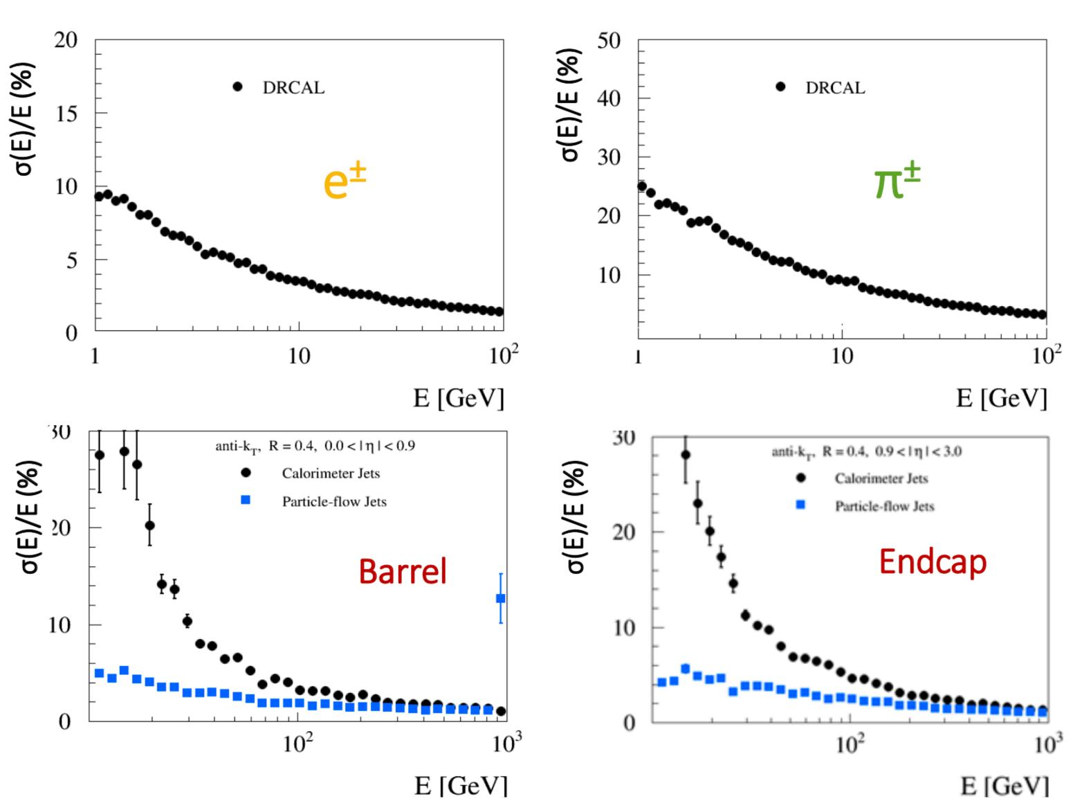
Energy resolution for reconstructed objects (both em and had particles) considering a  $\eta$  range with particle gun events (electrons and pions)
