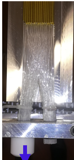
Cut edges of bunch of fibers inserted in a Teflon Container
