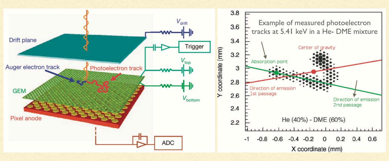
They are able to calculate the direction of a 5 keV e- in gas
