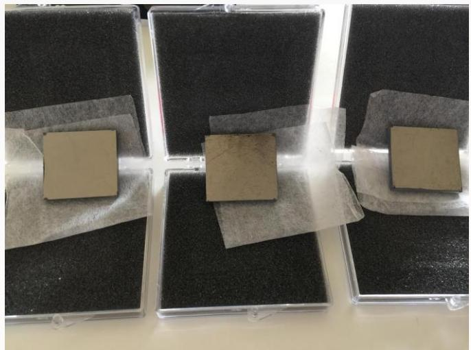
Set of different parameters HAPG crystals
