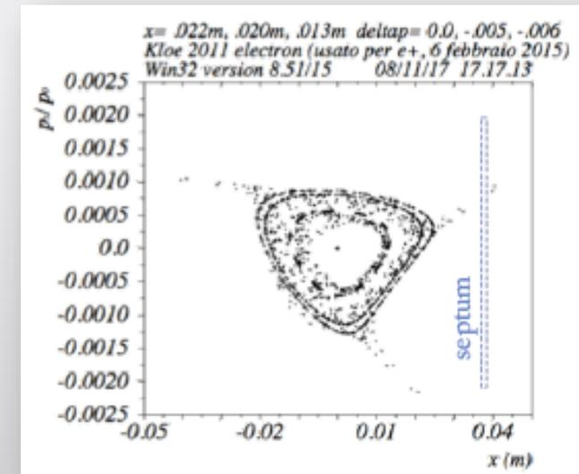
With **0.5% spread** at injection, wigglers **off**, expected pulse length of **0.42 ms**
