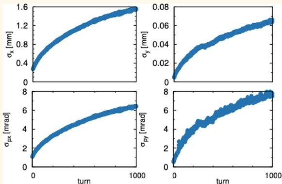
Beam evolution in the ring with 50 $\mu$ m Be target at IP
