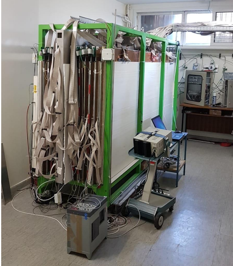
Avalanche RPC: strips readout by ALICE FEERIC ASICs, providing LVDS signals
