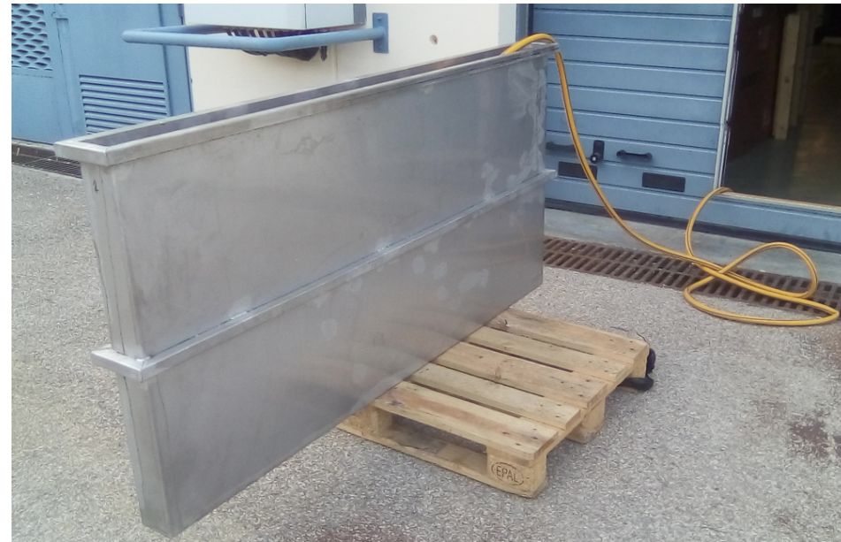
Leak testing with water
