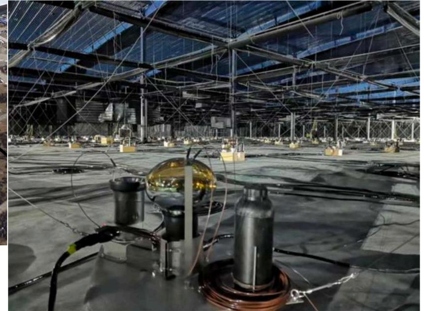
— > 1/4 of central Water Cherenkov detector operational (>HAWC size)
