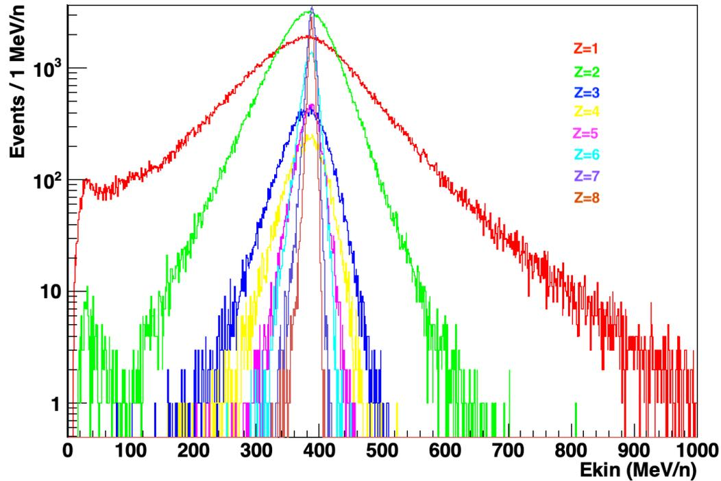
Asking for only primary fragments with origin in Target (over threshold) with production angle  $< 5.7^\circ$  and beam projection on TG in  $[-0.7, 0.7]$  matching a TW hit
