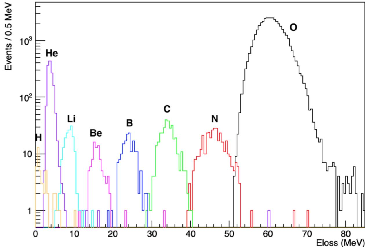
The combination of the Z identification and clustering algorithms implemented in SHOE provide a very good fragment charge identification on an event-by-event basis (DATA!!)
