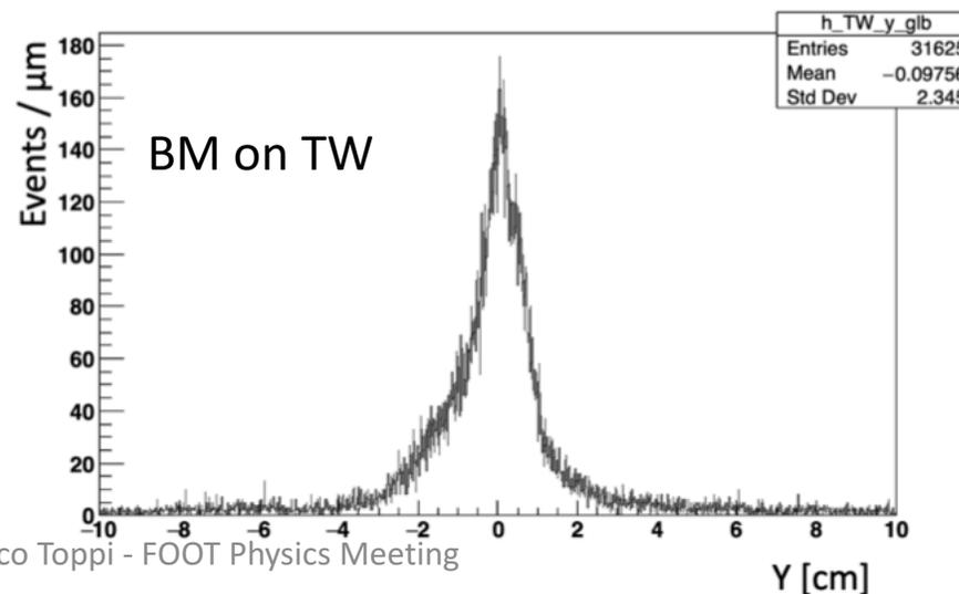
The broadening of the distribution on the TW shows a divergence of the beam of  $\sim 5$  mrad (about  $0.3^\circ$ ) in X and Y  $\rightarrow$  to be considered in systematics
