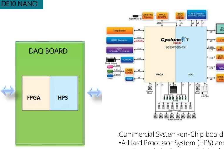
•A Hard Processor System (HPS) and an FPGA •Dual-core ARM Cortex-A9 & Intel Cyclone V FPGA
