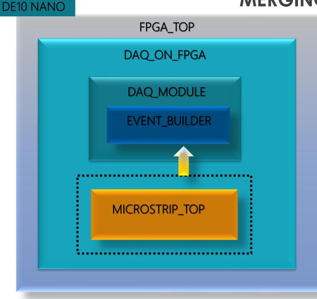
The microstrip\_top entity contains all the control signals to the ustrip detector interface and the logic to obtain and deliver the digitized data to the rest of the bologna group daq system.
