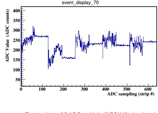
The readout of 5 ADCs, with half IDE1140 glued and bonded as shown in figure
