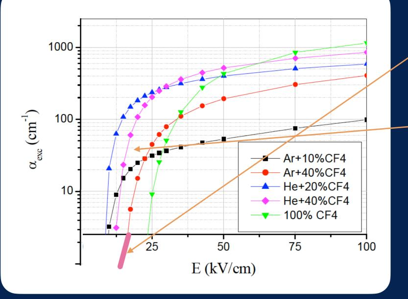
The increase of light production has a lower dependence on the Electric field than expected data do;
