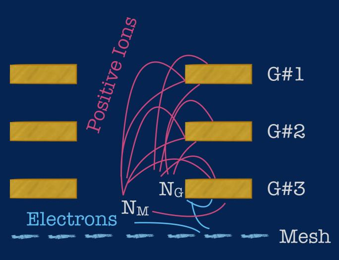
In general, we expect  $\Sigma_{tot} = 0$ and in particular  $I_M + I_{3D} = -(I_{3U} + I_{21})$ (equations are not independent) Let's assume all charges are produced in GEM#3 ( $N_G$ ) and, in case, in the gap above the Mesh ( $N_M$ );
