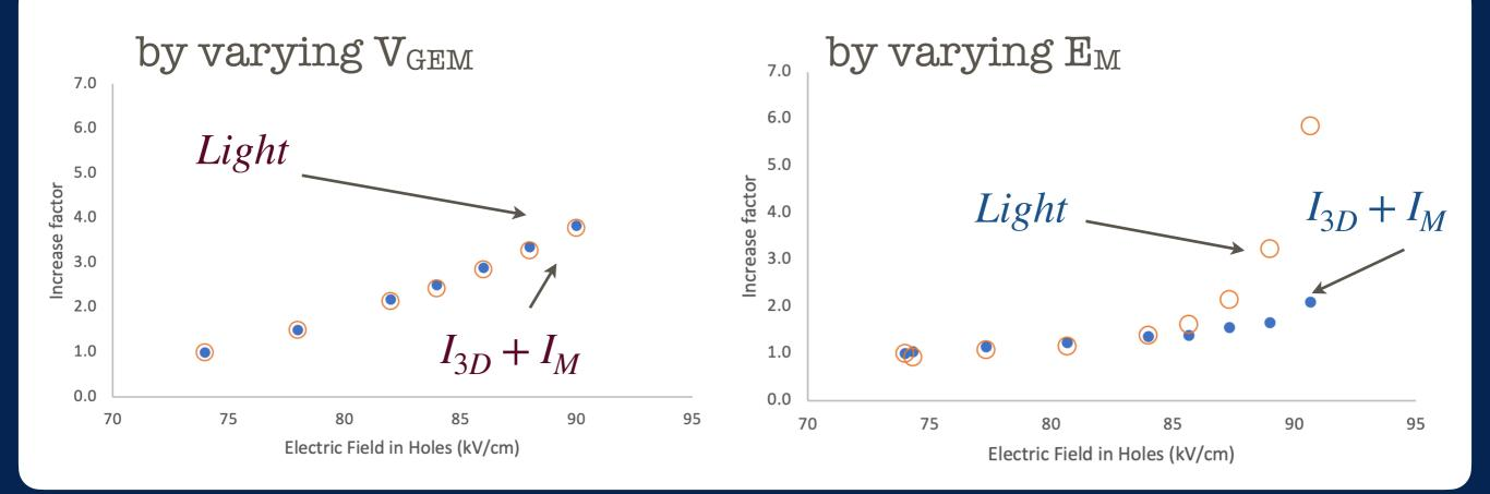
When increasing  $V_{GEM}$  light and current have the same behavior; Effect of the  $E_M$  seems completely different;
