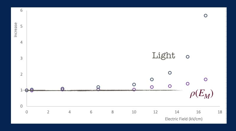
For electric fields larger than 10 kV/cm,  $\rho(E_M)$  starts to be significantly different from 1
