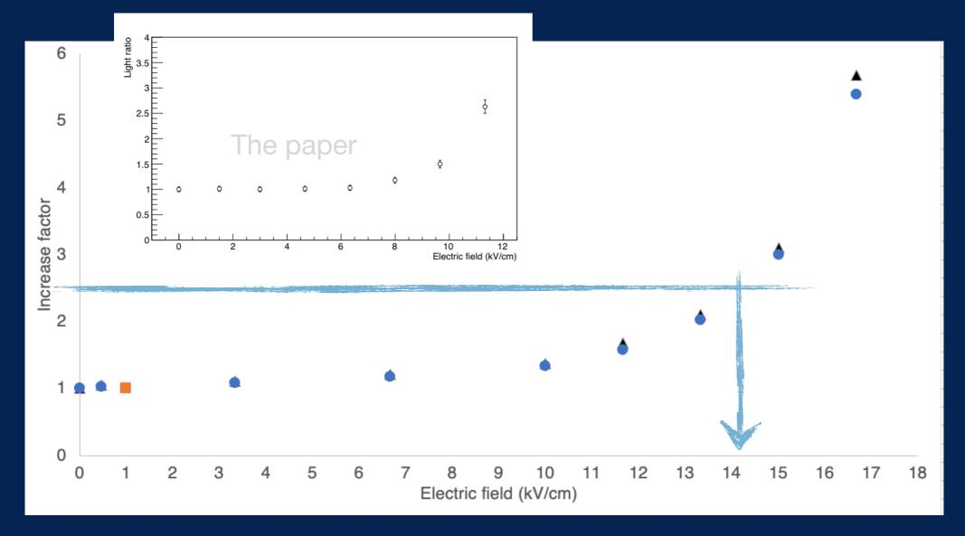
In order to get a light increase of a factor 2.5, a field of about 14 kV/cm is needed;
