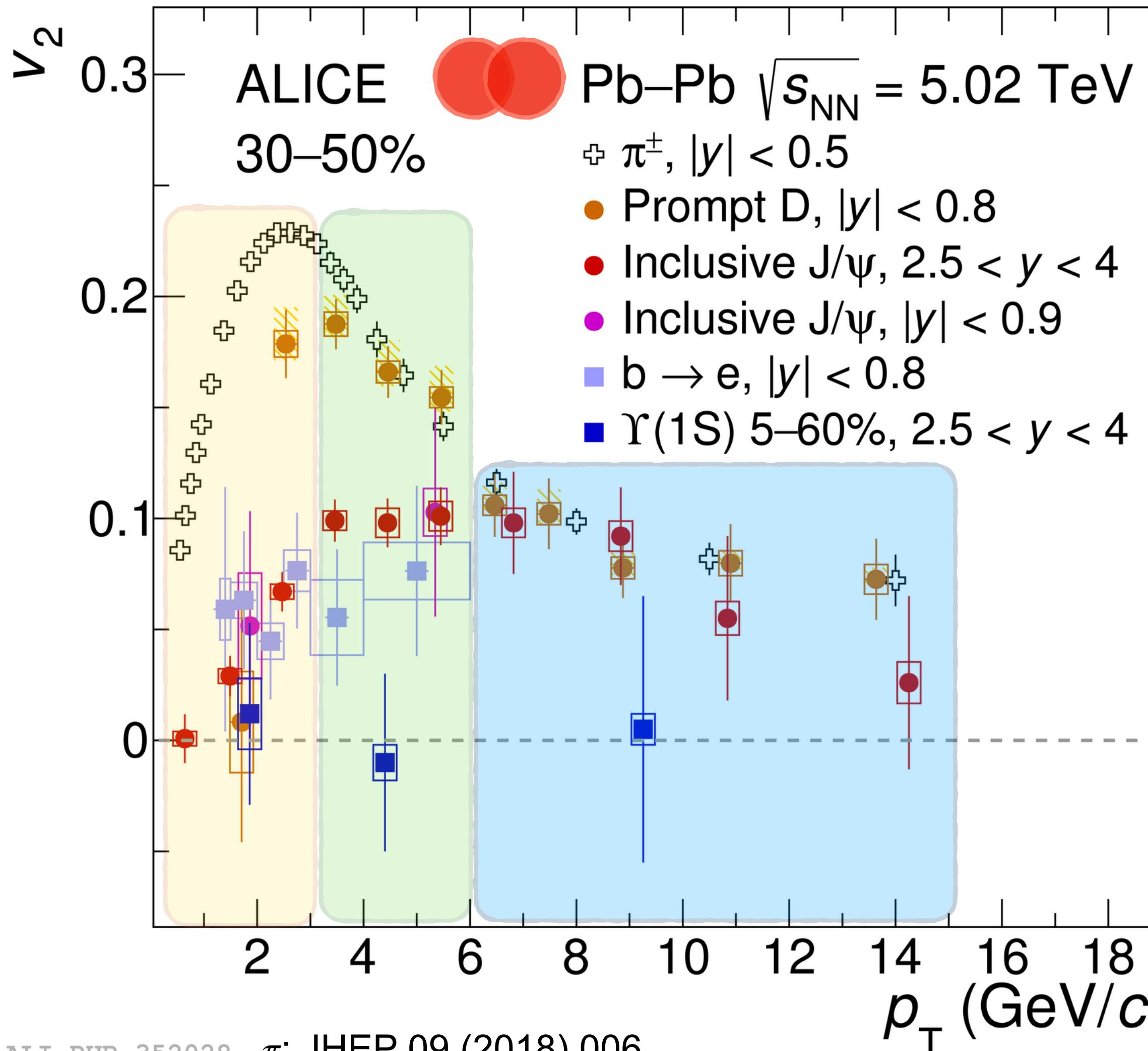
$$p_T < 3 \text{ GeV}/c \Rightarrow v_2(\text{J}/\psi) < v_2(\text{D}) < v_2(\pi^\pm)$$
