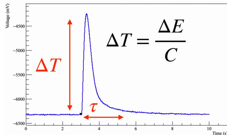
Pulse amplitude  $\propto \Delta T \propto \Delta E$
