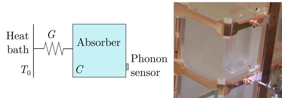
Particle energy release measured via crystal temperature increase
