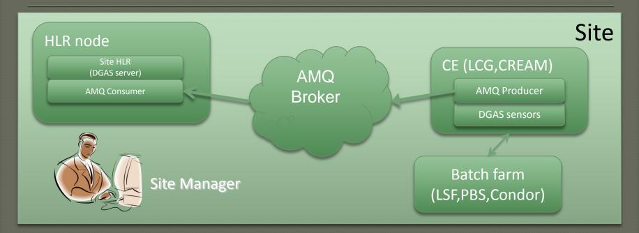
With the Active MQ model, the sensors act as message producers, while the HLR is a message consumer. In this scenario it is not possible to use an encrypted communication channel, so encryption is performed on a per-message basis.
