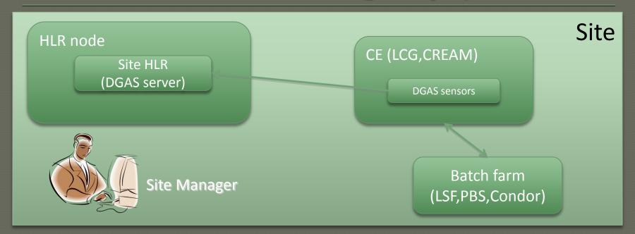
The basic, legacy, DGAS communication protocol is based upon a client-server infrastructure, with a double commit push protocol based on a GSS over TCP secured channel.
