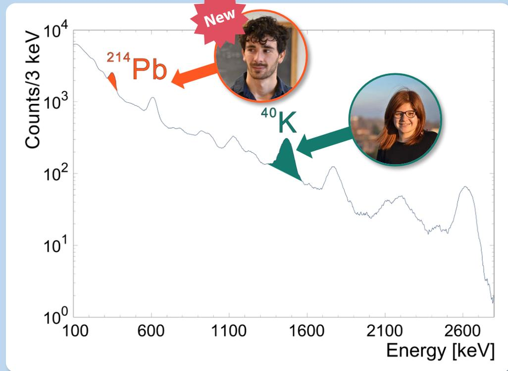
$^{40}\text{K}$  and  $^{214}\text{Pb}$  emit  $\gamma$ -rays that can be sensed by spectroscopic stations
