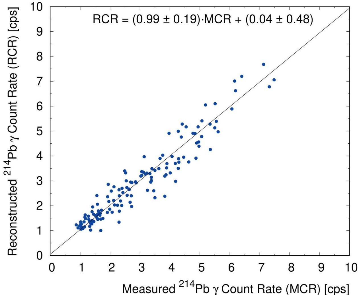
The reliability of the model is demonstrated by the **good linear relation** observed between **measured** and **reconstructed  $^{214}\text{Pb}$**  net count rate during the rain time.
