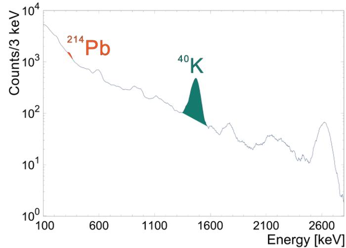
During a rainfall, the **soil water content  $w$**  can still be estimated by the attenuated  $S_K$  signal.
