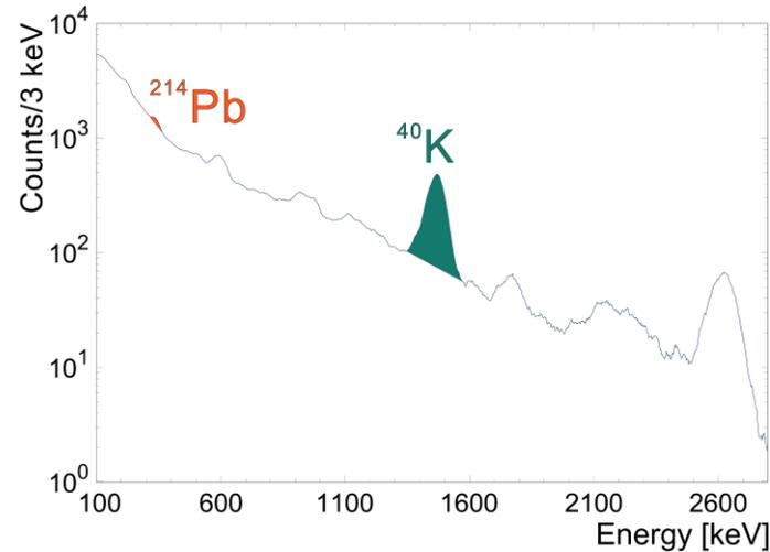
After an irrigation, the  $\gamma$  signal is **attenuated** by the **water deposited** between the emitters (i.e. the **soil**) and the detector.
