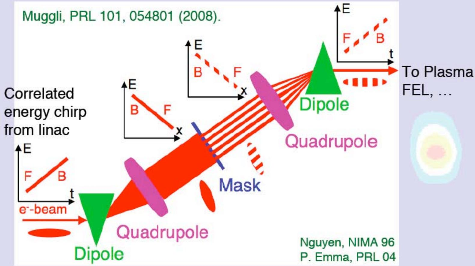
➔ Choose microbunches spacing and widths with mask and beam parameters:  $N$ ,  $\Delta z$ ,  $\sigma_z$ ,  $Q$
