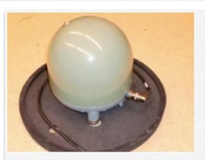
The seismometers are usually mounted on a hardrock tile (attached to the ground with concrete) and covered by an acoustic insulating cover. A thermal insulating box filled with insulation foam is then placed on top of the instrument to further isolation the instrument from external influences.
