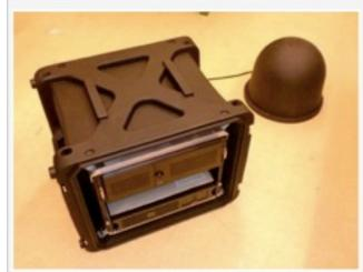
Data acquisition unit with seismometer in acoustic cover
