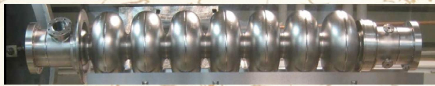
ERL Linac based on SC cavities operating in CW challenges: **Minimize RF power dissipation for design E**<sub>acc</sub> **Beam instability and beam breakup HOM excitation and extraction Microphonics High gradient stability**
