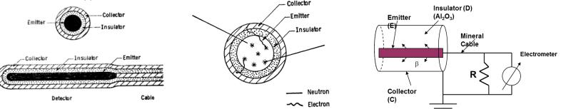
V, Co, Rh are common elements used as emitter in the thermal neutron SPNDs. Their sensitivity for fast neutron is rather low due to limited cross section of these elements. Alternative materials should be used to cover fast neutron energy range.
