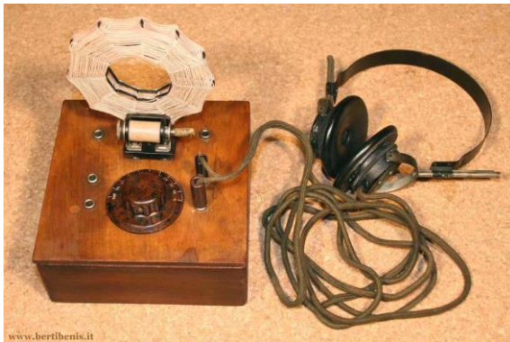
Crystal radio – 1906 Self-powered by radio waves
