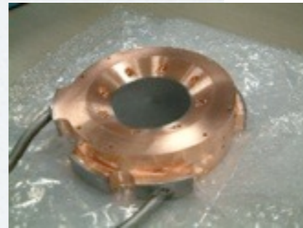
Graphite target with water cooling
