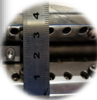
Inner diameter of undulator vacuum box ~4 mm
