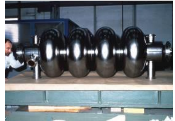
Radiofrequency cavity (1 m-long)
