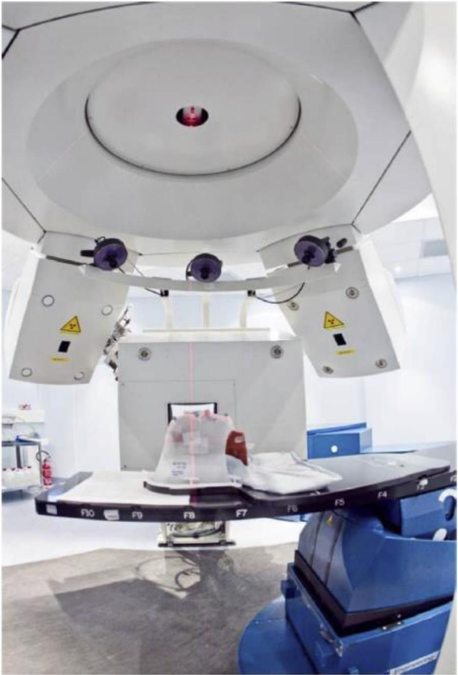
**Figure 14.** Patient positioning and verification systems inside one of the treatment rooms at CNAO.
