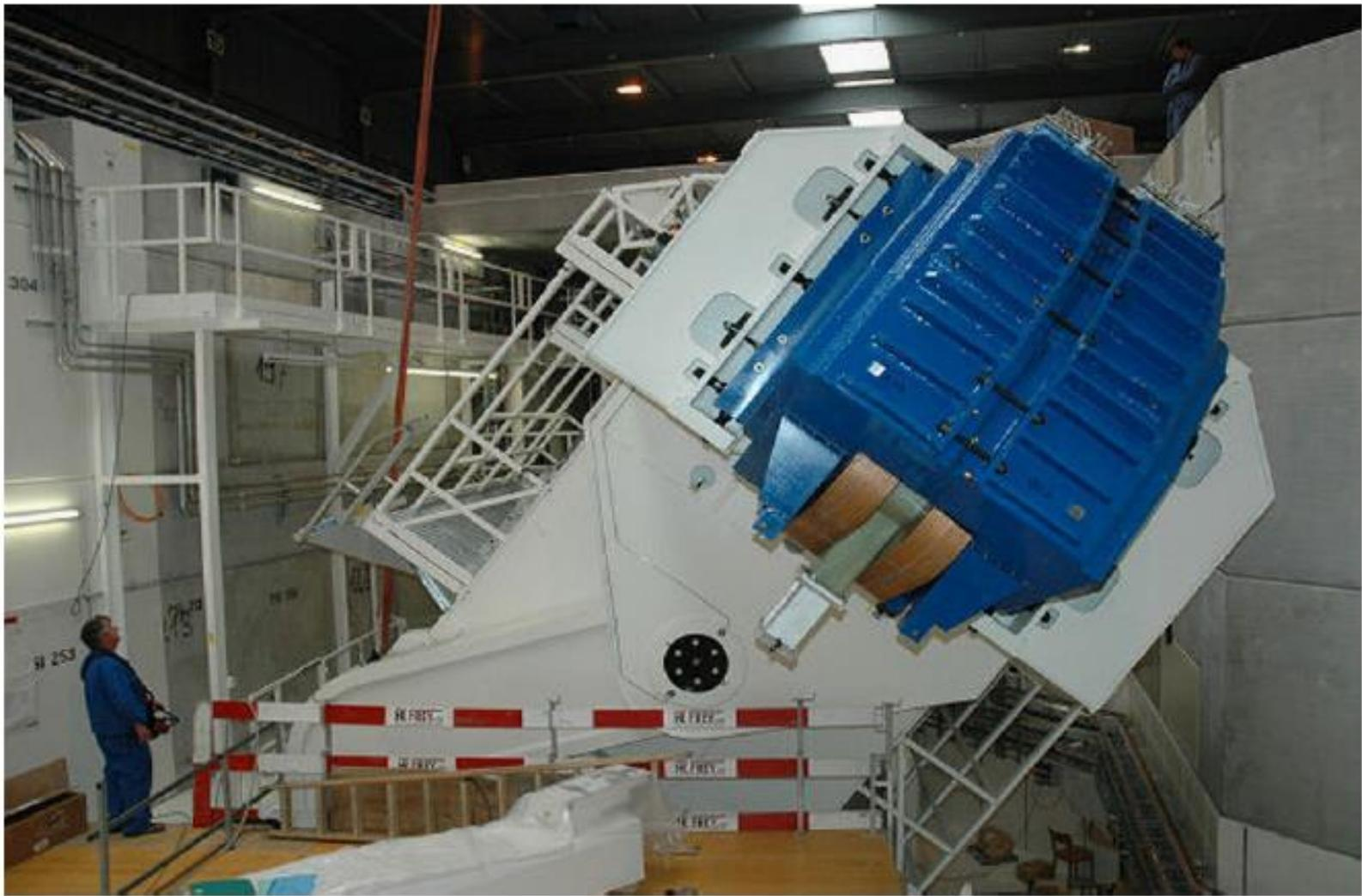
**Fig. 7.** Installation of the Paul Scherrer Institute Gantry 2, which utilises scanning magnets upstream of the final dipole in a Pavlovic-style optics also used at HIT but not commonly in other centres. Parallel beam scanning is enabled at the expense of a larger, more complex final bending magnet.
