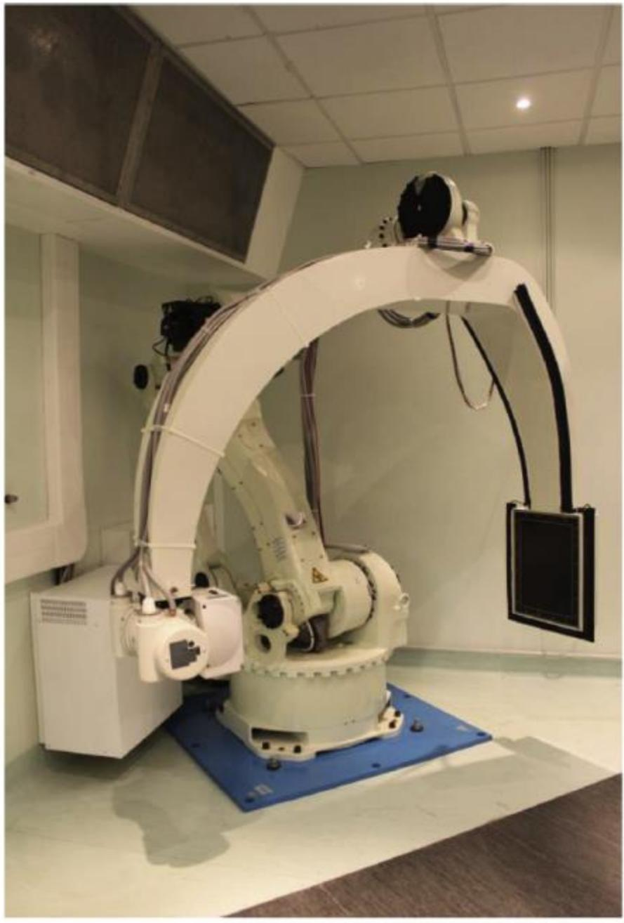
**Figure 15.** The custom robotic in-room imaging installed in the central room of CNAO.
