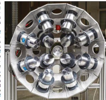
Future view Atomki's new high-resolution LaBr 3 spectrometer, which will record gamma-gamma pairs from excited nuclei.
