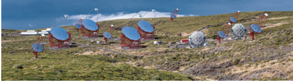
CTA North (La Palma island, Spain): 4x LST (23m) + 15 x MST (12m)
