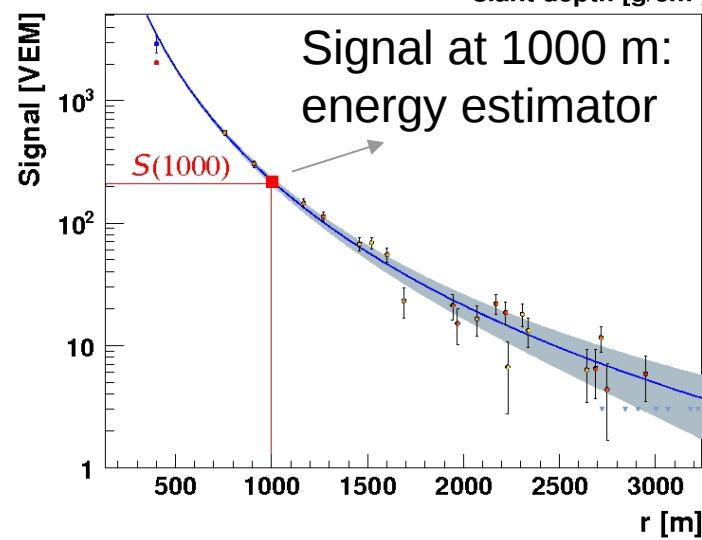
Use the energy scale provided by FD to calibrate the entire SD data sample
