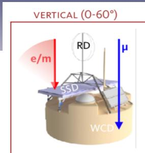
Scintillators are sensitive to the electromagnetic content of the shower
