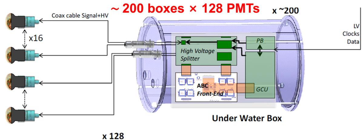
Under water box provides supply for 128 PMTs
