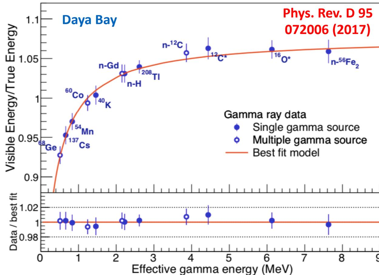
Ratio of observed energy to true energy for  $\gamma$ -rays
