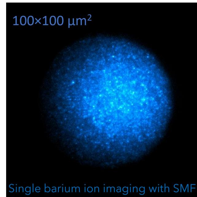
On/off molecules: dry single-molecule imaging with TPC-compatible microscopy
