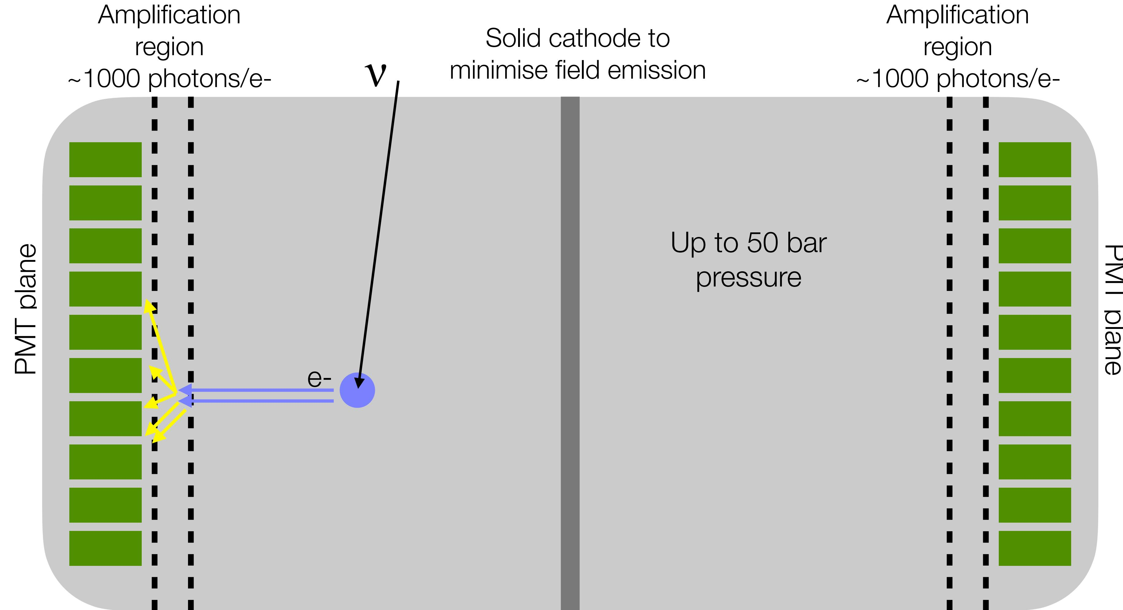
Symmetric detector with two PMT planes to be sensitive to tiny signals.
