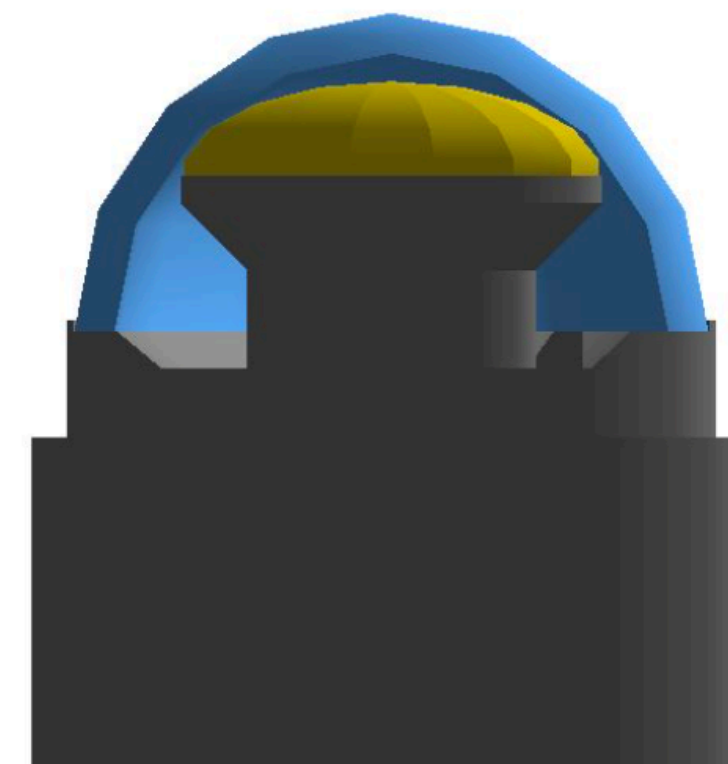
SDOM PMT housing Geant4 model
