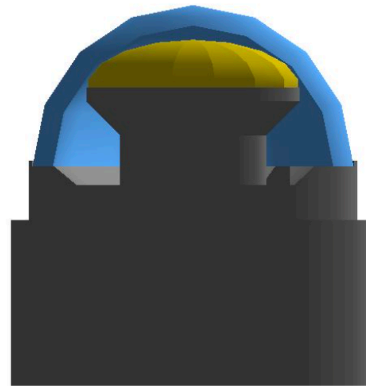
SDOM PMT housing Geant4 model
