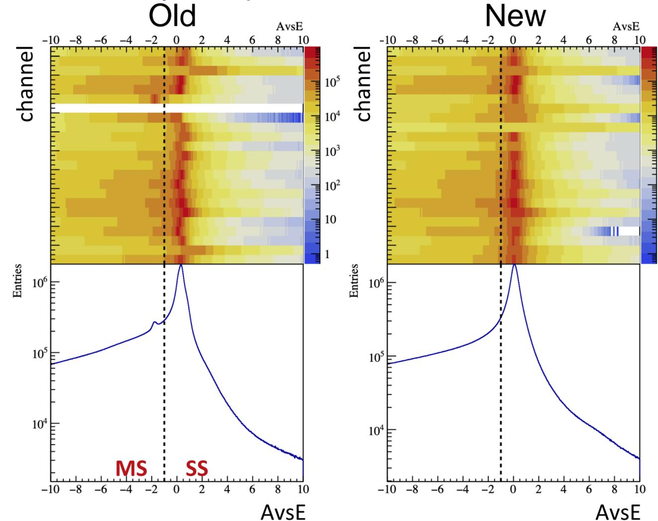
The new AvsE parameter offers better stability and uniformity across all detectors, while accounting for acceptance degradation at higher energies. The result is a better multi-site discriminating parameter
