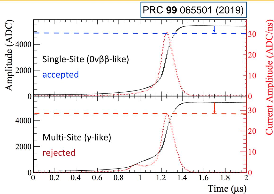
Amplitude of current pulse is suppressed for a multi-site event compared to a single-site event of the same event Energy (AvsE)
