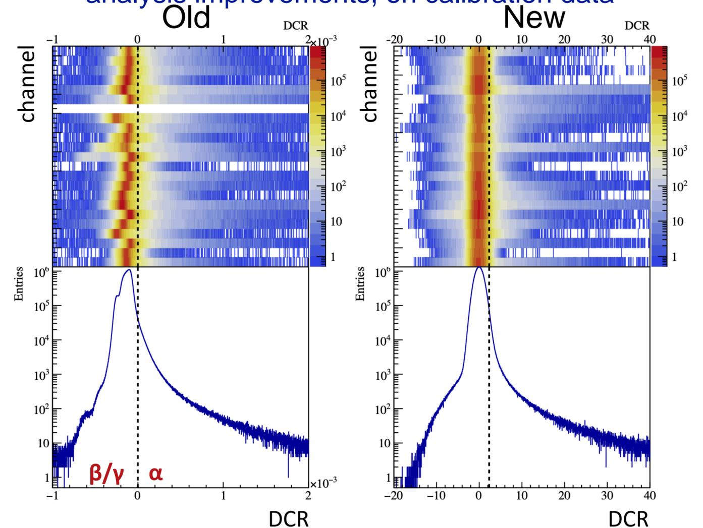
The new DCR parameter provides better stability across time and across detectors as well as increased exposure. Better discrimination between normal bulk events and alphas is expected.
