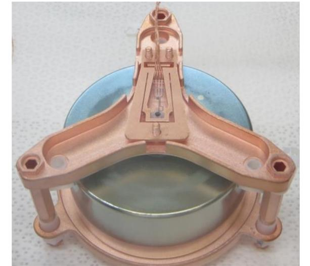
Array components and passive shielding fabricated from ultra-pure materials with extremely low radio-isotope content
