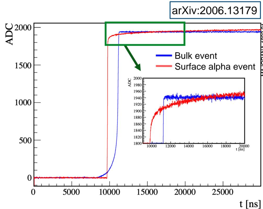
Alpha penetrating passivated surface result in trapped charge that is slowly released into bulk: delayed charge recovery (DCR) measured via slope of flat-top
