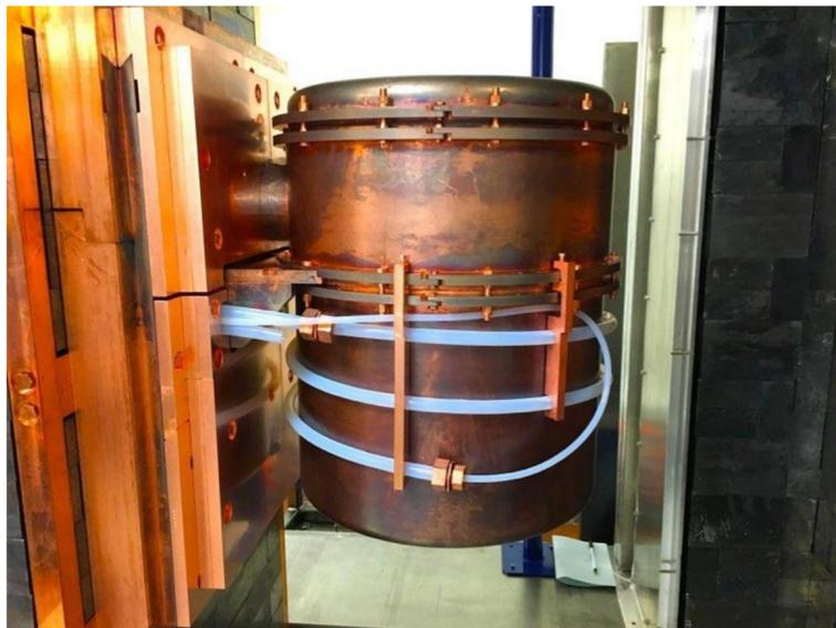
$^{228}\text{Th}$  calibration line source is placed in tubing surrounding cryostat
