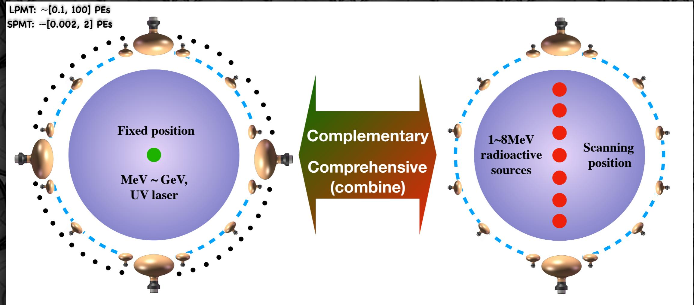
Direct calibration of potential QNL of LPMT at every single channel level for JUNO reactor neutrino physics
