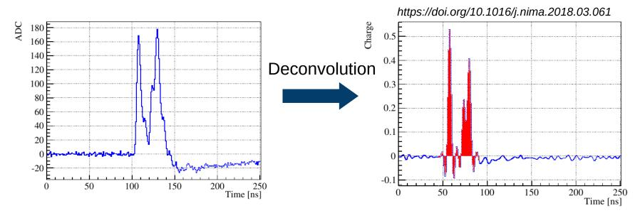
Other methods: waveform fitting, simple charge integration, etc.
