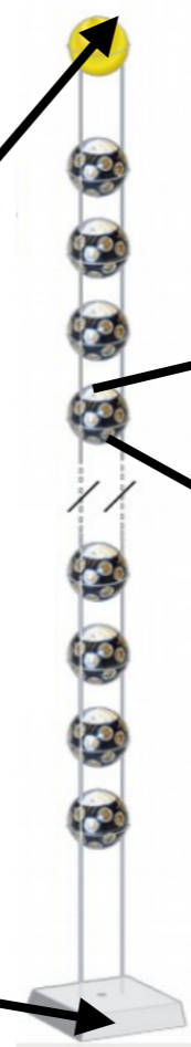
Detection Unit (DU) aka "string/line"
