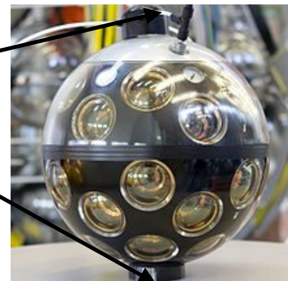
KM3NeT DOM housing 31 3" PMTs
