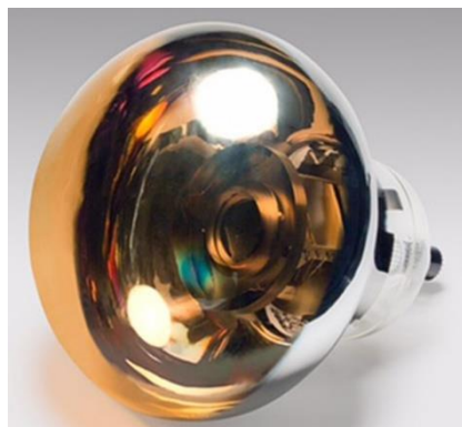
5000 dynode PMTs type Hamamatsu R12860
