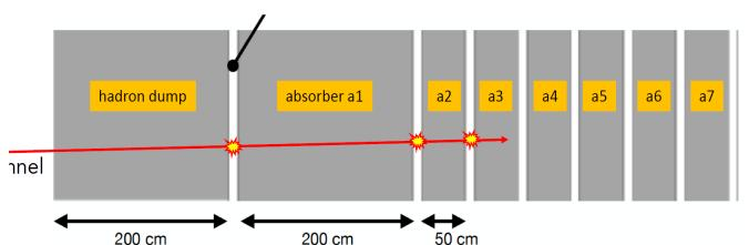
Muon range-meter in the hadron dump: in progress
