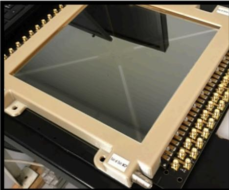
Micro-channel plate, fast-timing photodetectors
