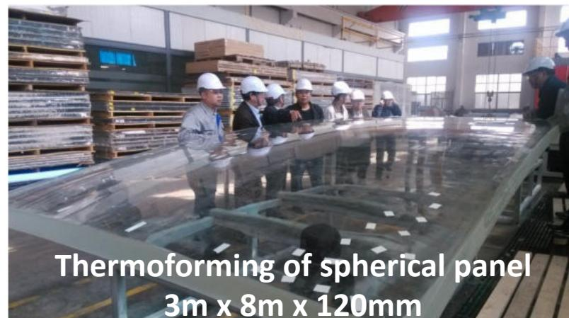
Thermoforming of spherical panel
