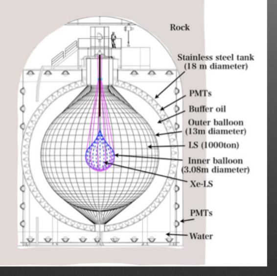
The inner balloon is filled with <sup>136</sup>Xe dissolved in liquid scintillator
