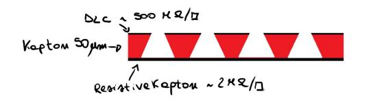
Amplification layers made of:
