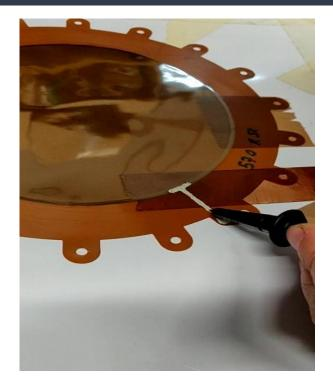
The conducting paste seems to have pierced the kapton foil  $\rightarrow$  there's a short that we couldn't see with the tester but we can observe here with the megger
