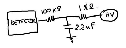
HV filter mounted on each HV channel
