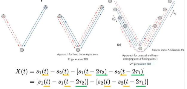
$s_i(t) = \text{laser phase in arm } i$
