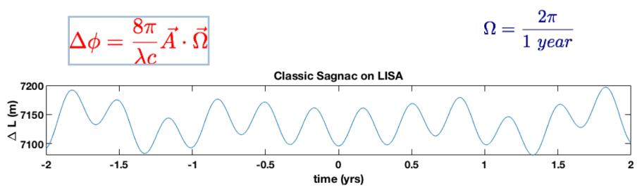
A large  $\Delta L$  with small oscillations due to breathing and flexing of the constellation (Keplerian changes in size and angles)
