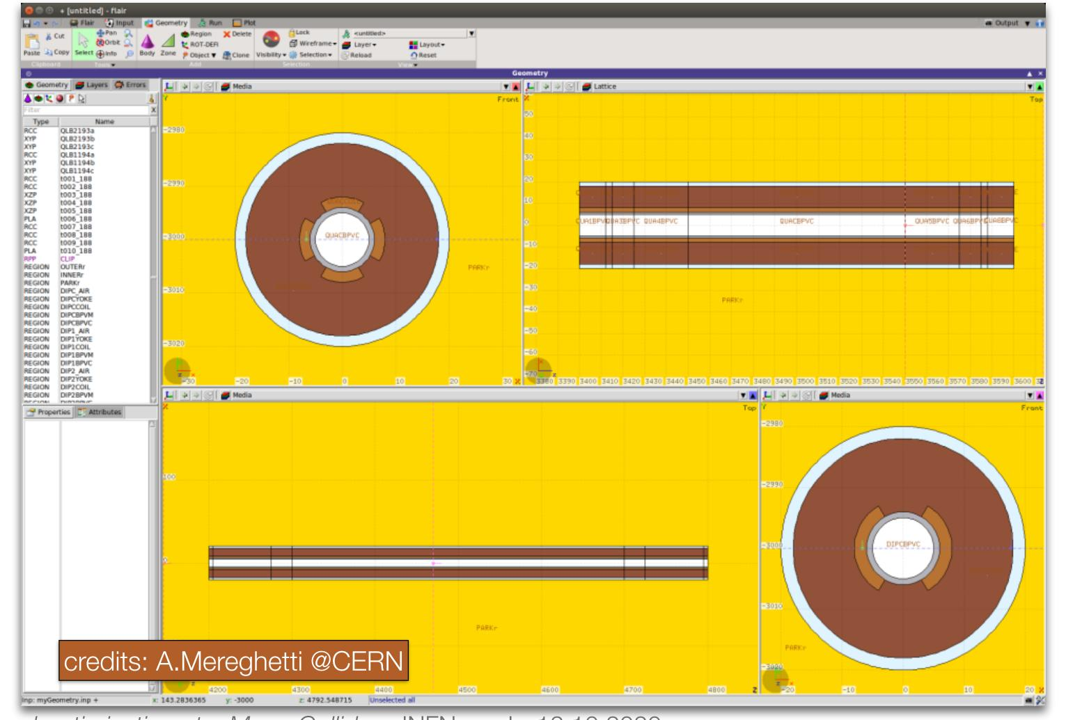
• The detector (w/ nozzle) has been added to the geometry (via an automatic script working on its .gdml file)
