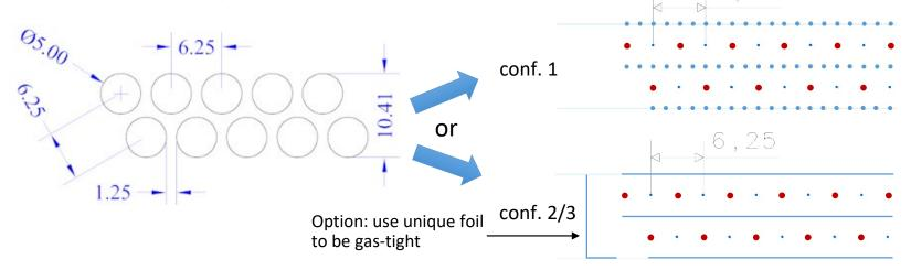
Simple construction (as used for MEG-II drift chamber):
