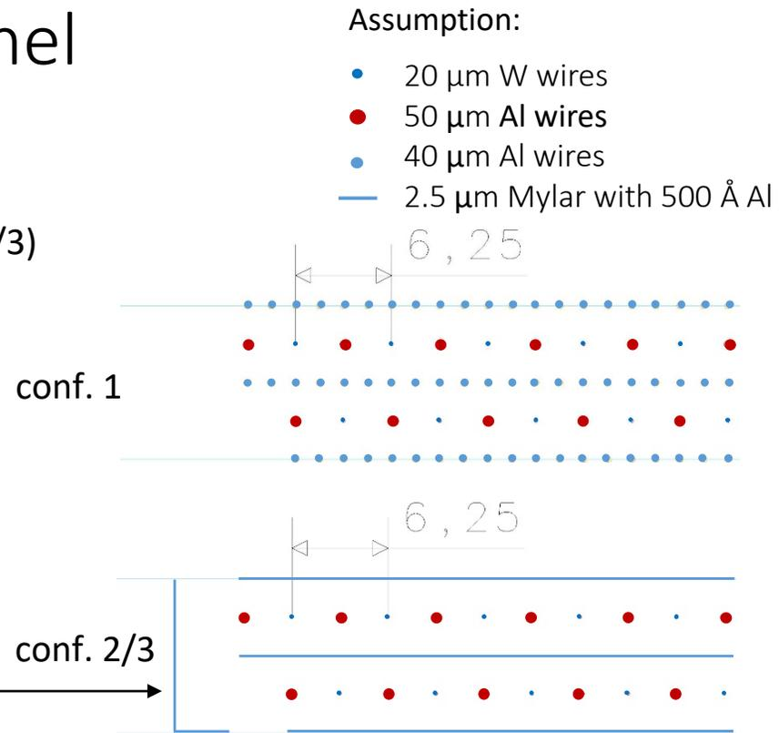
Simple construction (as used for MEG-II drift chamber):
