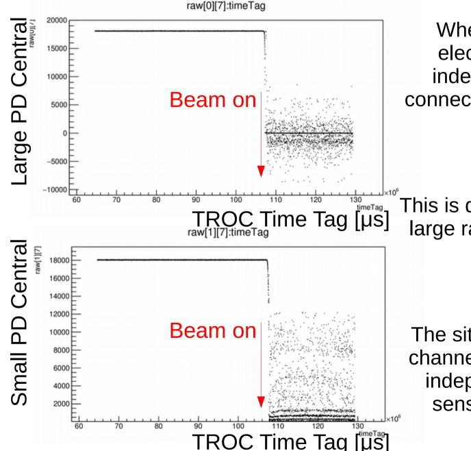
When the beam is on, the electronics stops to work, independently if the chip is connected to large or small PDs.
