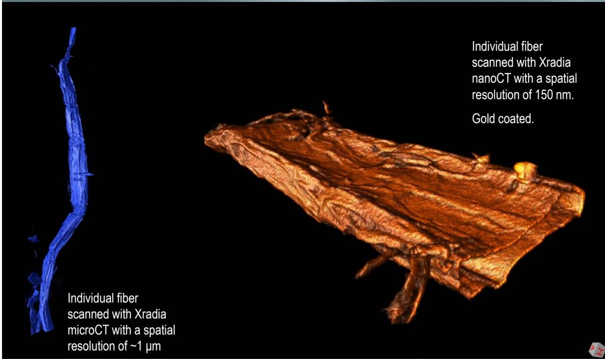
Individual fiber scanned with Xradia nanoCT with a spatial resolution of 150 nm.
