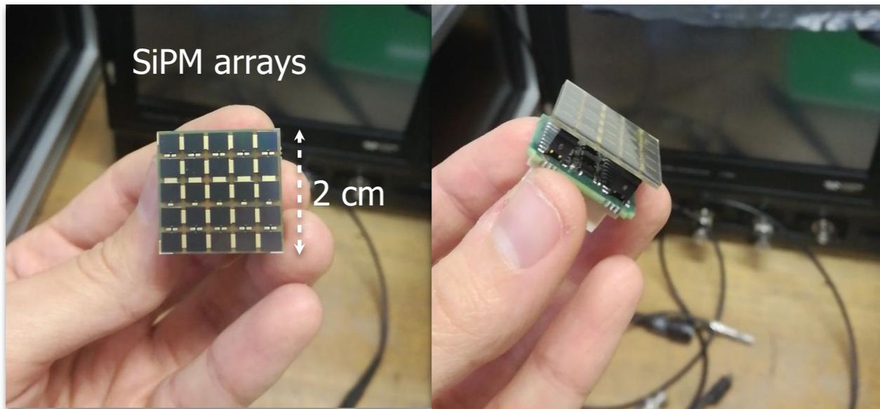
SiPM arrays with 15 $\mu$ m size of microcells
