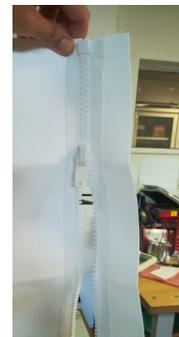
Zipper to close the ePTFE reflectors around the pipes
